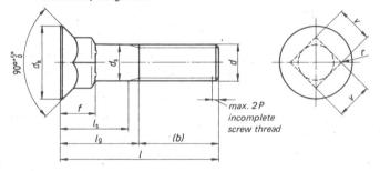
Designation of a flat countersunk square neck bolt with short square, with screw thread d=M 10, length l=50 mm and strength category 3.6 or 4.6 (at manufacturer's discretion):
